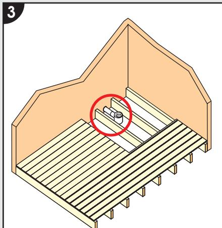
Fit waste pipe and trap making sure it will align with the centre of the gully aperture in the level-dec.
