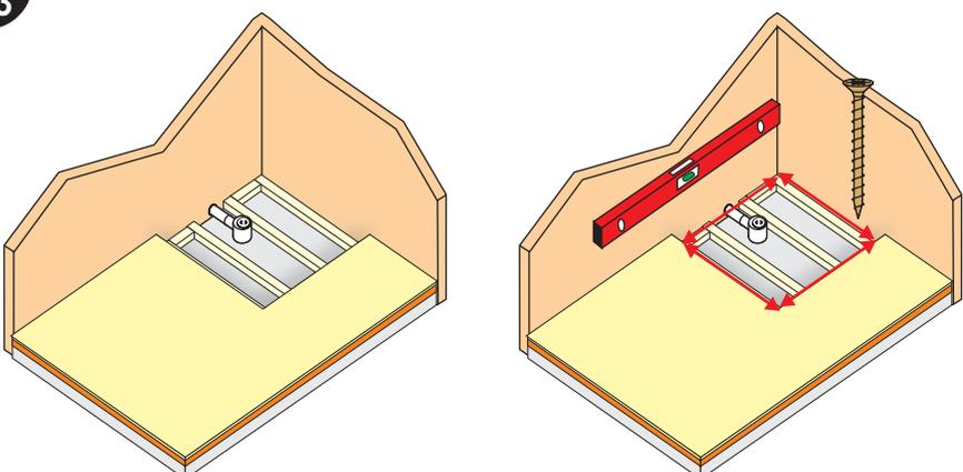
Fit timber support to prevent the edge of the chipboard flooring from moving and to provide a firm foundation for the level-dec.
