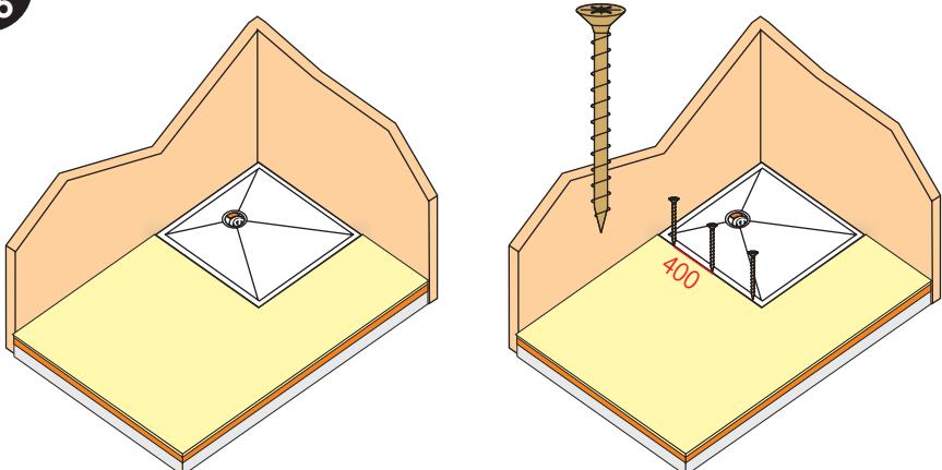
Put Dec into position drill and counter sink holes for the 4x60mm screws.
