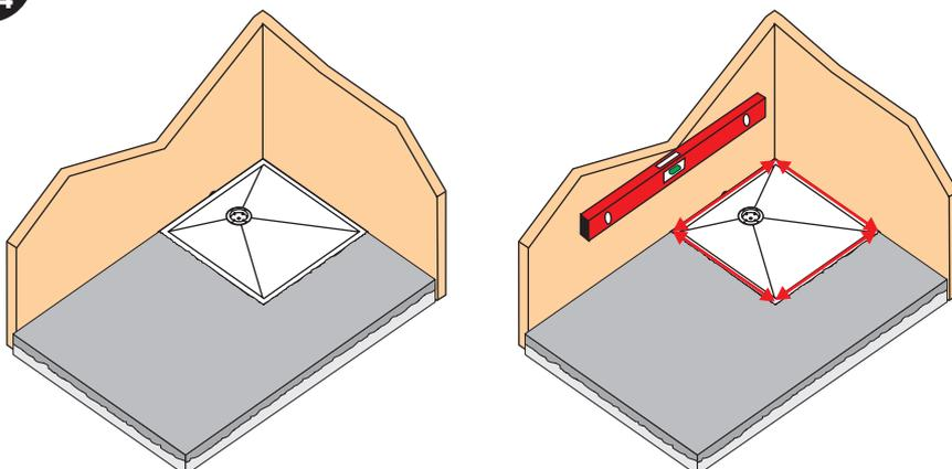
Place Dec into position and check accurate positioning of the waste
