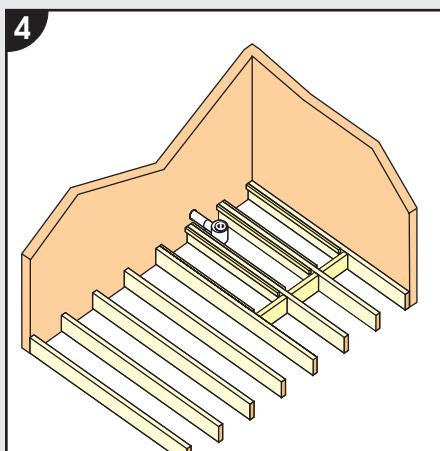
Screw battens to the joists leaving enough room between the top of the batten and the top of the joist for the 18mm plywood.
