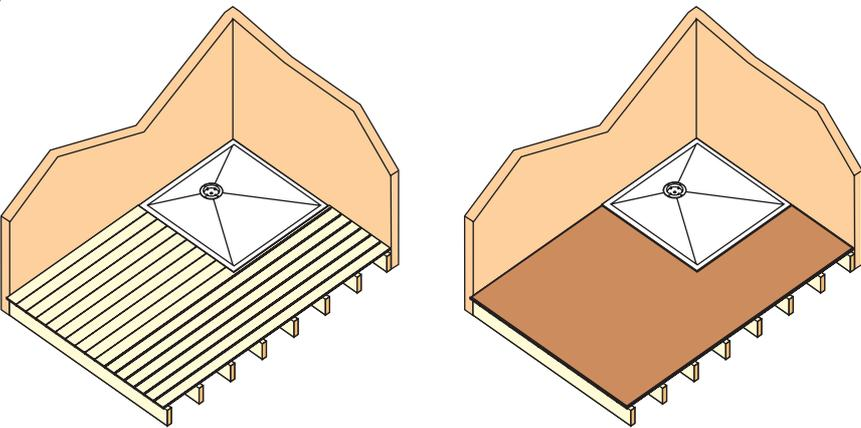
It may be necessary to put plywood over the rest of the floor to make it level with the Dec.
