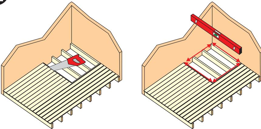
Carefully cut out line and remove the floorboards.
