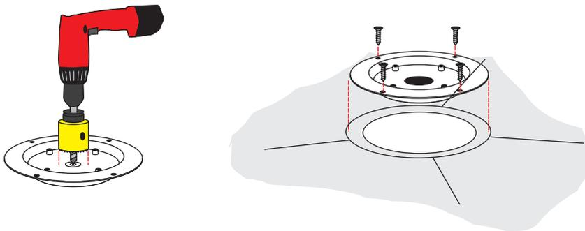
Drill out the centre of the trap-a-dapta (base) with a 50mm holesaw.
