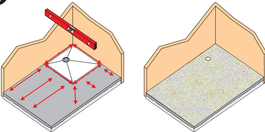
Finally check that the Dec is level on all 4 sides.
