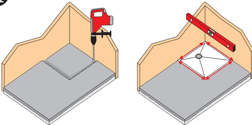
Excavate all concrete within the marked area to a minimum depth of 25mm.
