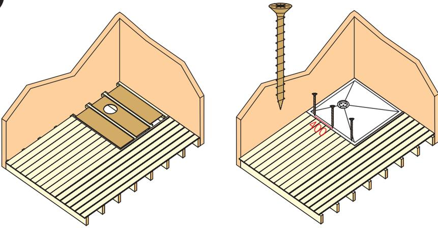
It may be necessary to apply expanding foam or silicone to the joists to take out any inconsistency in level.
