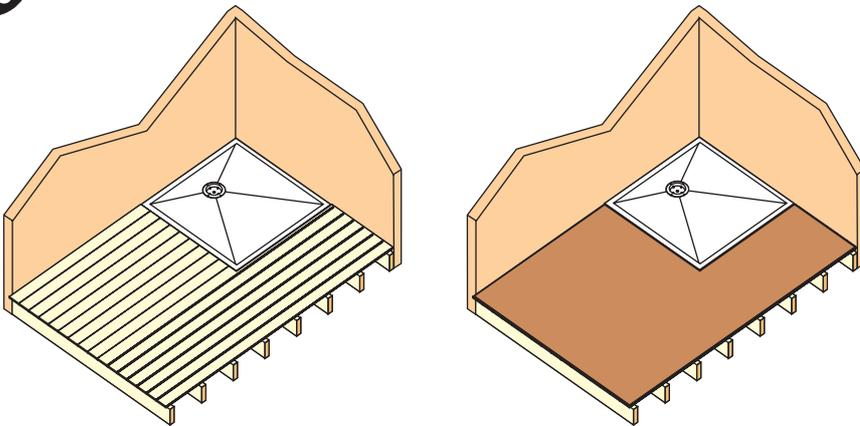
It may be necessary to put 4mm plywood over the rest of the floor to make it level with the Dec.
