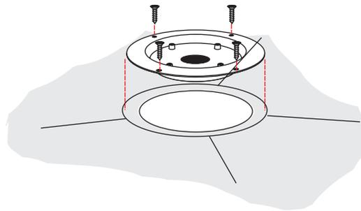
Drill out the centre of the trap-a-dapta (base) with a 50mm holesaw.
