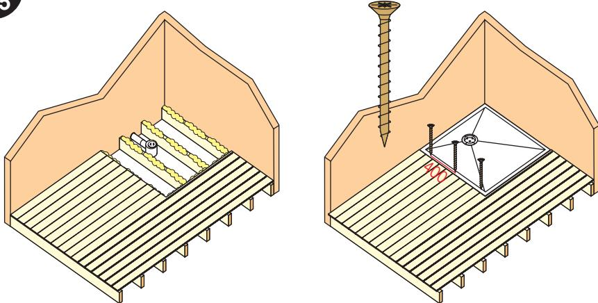
It may be necessary to apply expanding foam or silicone to the joists to take out any inconsistency in level.
