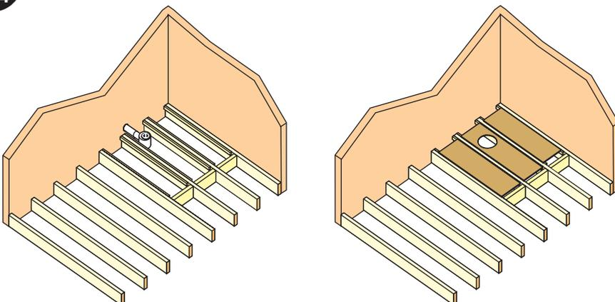
Screw battens to the joists leaving enough room between the top of the batten and the top of the joist for the 18mm plywood.
