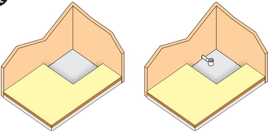
Carefully cut out and remove chipboard flooring, vapour barrier and insulation.
