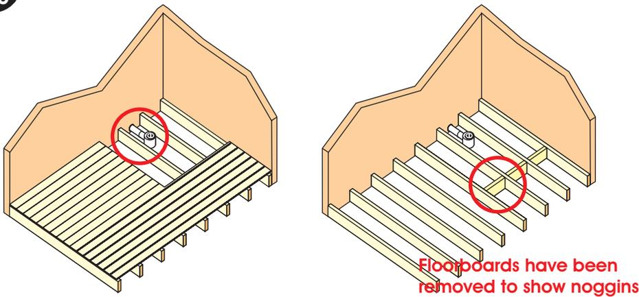
Fit waste pipe and trap making sure it will align with the centre of the gully aperture in the level-dec.
