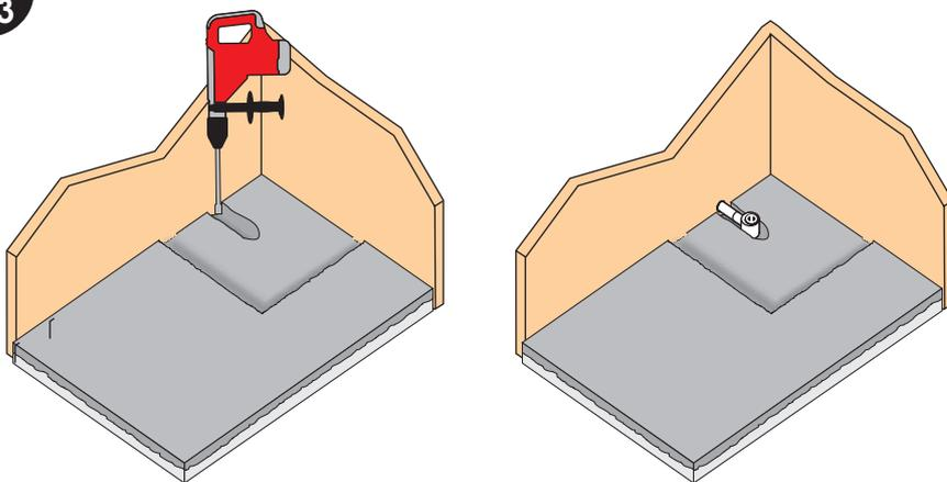
Remove enough concrete for the installation of a waste pipe and gully.
