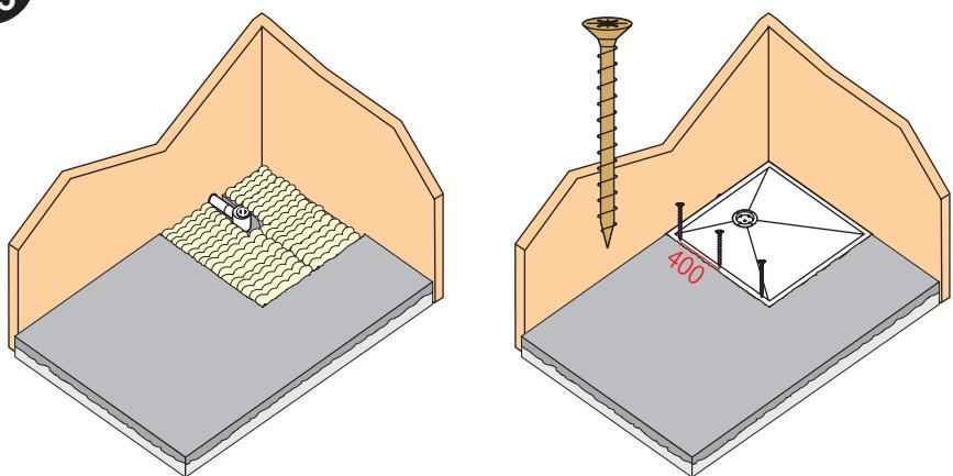
Bed the tray on a weak sand cement mix or expanding foam.
