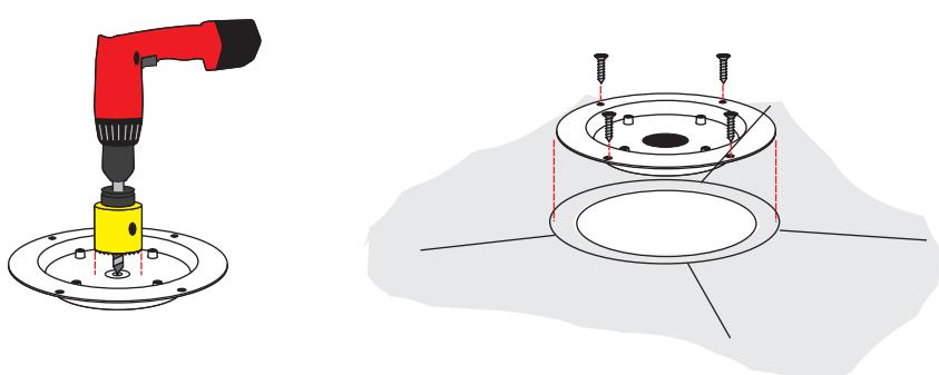
Drill out the centre of the trap-a-dapta (base) with a 50mm holesaw.
