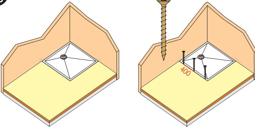
Put Dec into position drill and counter sink holes for the 4x60mm screws. Drilling at a maximum of 400mm centres around the perimeter of the Dec.
